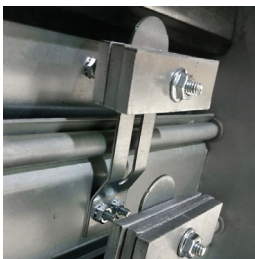
counterbalance weights mounted to blades
