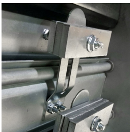
counterbalance weights mounted to blades
