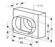
W = Width (Duct) H = Height (Duct) X = Variable (See Size Chart) D = Diameter
